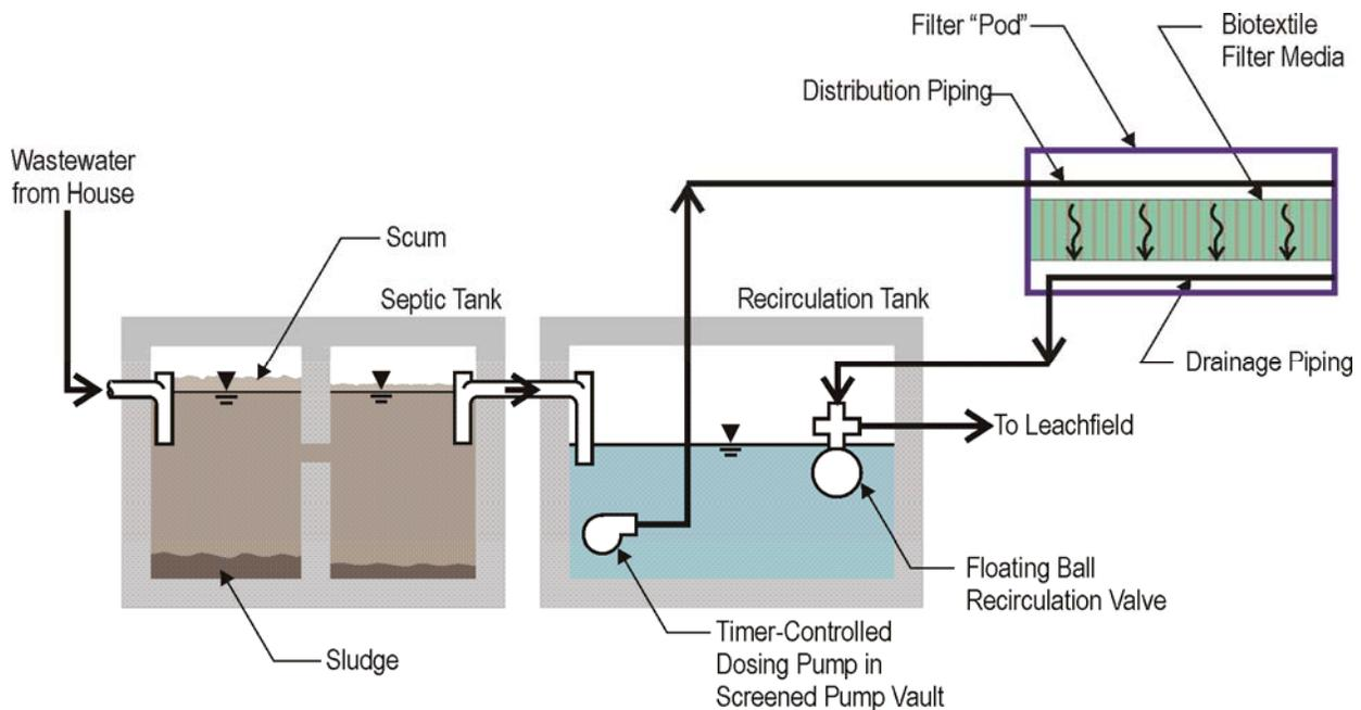
Biotextile filters have proven to produce excellent quality effluent when compared with typical septic tank effluent, as shown in Table 6-6. The table shows that biotextile filter effluent contains significantly less biochemical oxygen demand and total suspended solids than typical septic tank effluent, which reduces solids and
