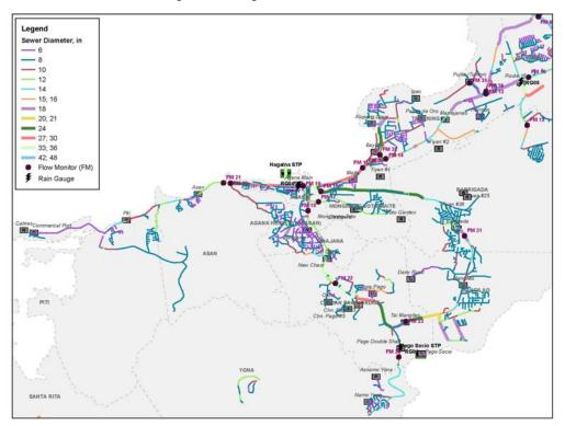
Figure 4-2 – Hagatna STP Sewer Network
