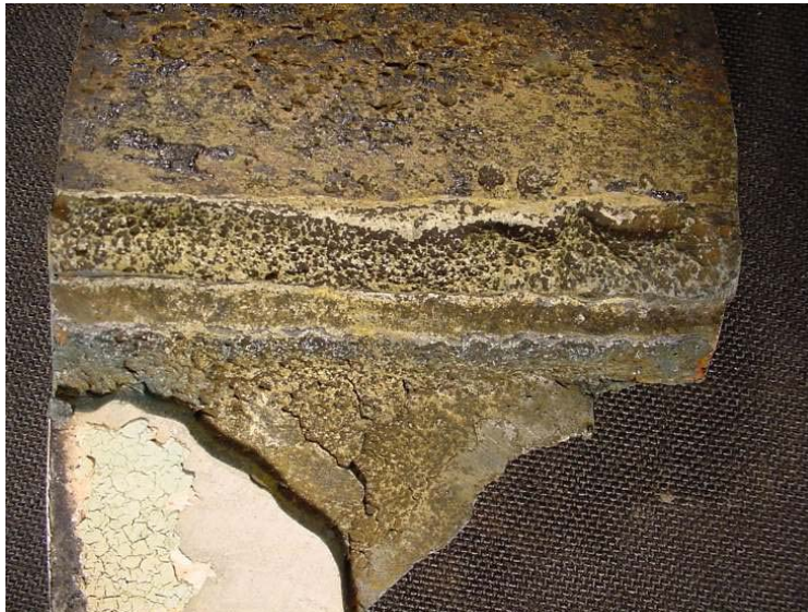
Figures 3 & 4 Show the samples after cleaning in an inhibited hydrochloric acid solution.
